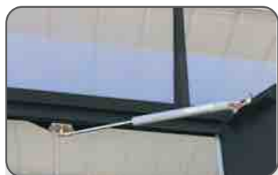
Hydraulic Shock to Keep Door Open
